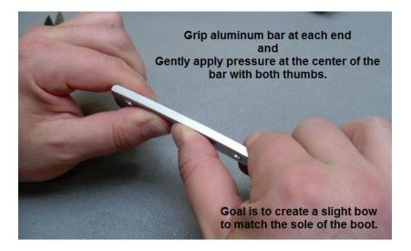
Once the bars have been slightly bowed to mirror the sole of the shoe, the bars can be attached using the screws and Loctite- blue 242.
