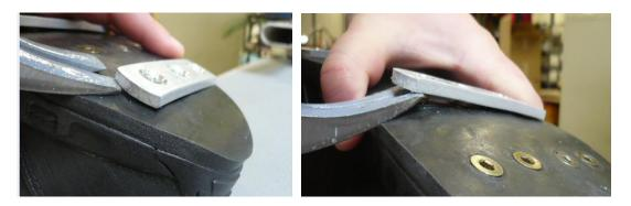
Gently pry the bar in upward motion, moving along the bar toward the opposite side of the shoe.
