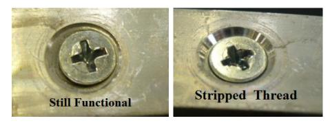
The stripped thread screw will then need to be pulled out with a claw hammer.
