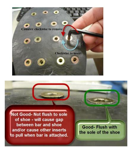
The inserts need to be as flush to the sole as possible. (Prevents any small debris from catching in the Aluminum Bar)
