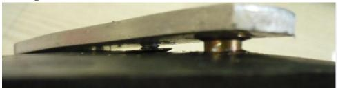
Insert the claw end of the hammer at the end of the bar where there is space between the sole and the bar.
