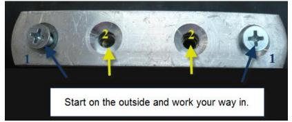
Once all screws have been inserted and bar is securely attached to the shoe. Repeat the steps for the remaining bars that need to be replaced.
